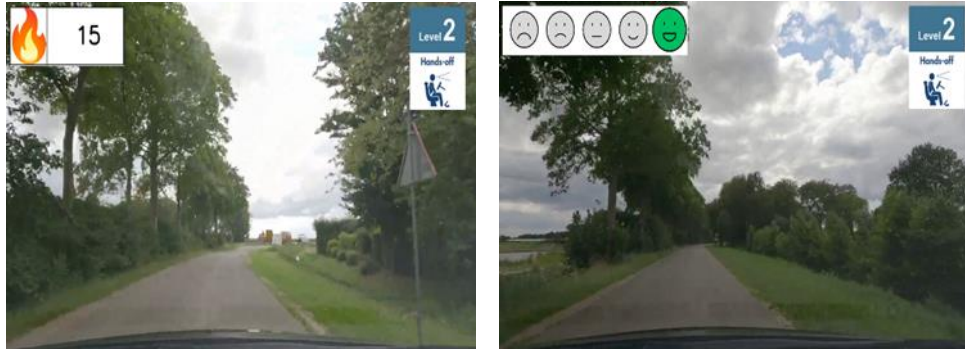
Fig. 3. Visualization of the gamification concept 4 . The authors developed two different feedback systems: one in which credit points could be accumulated, where the points drop to zero at the first miss use and another in which a positive smiley was displayed for correct behaviour, but which was gradually downgraded for non-level compliant behaviour.
