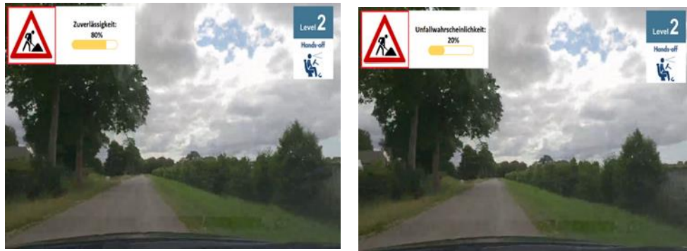
Fig. 2. Visualization of the trust calibration 3 . In the visualization, a schematic representation of the traffic situation is presented to the driver, with the aim of conveying the information in a transparent way. The authors developed a variant that indicates reliability and another that indicates the probability of an accident.
